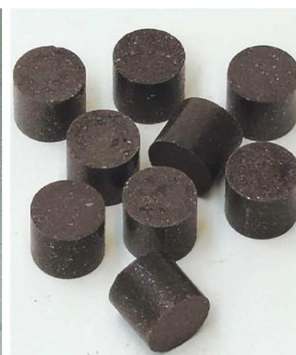
Agglomeration trials with tablet press
