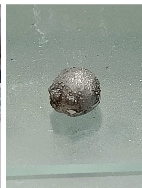
TransZeroWaste hot microwave pelletising with reduction potential
