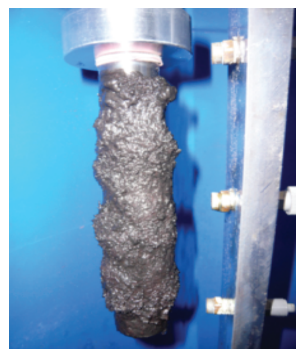
Magnet loaded with oily scale
